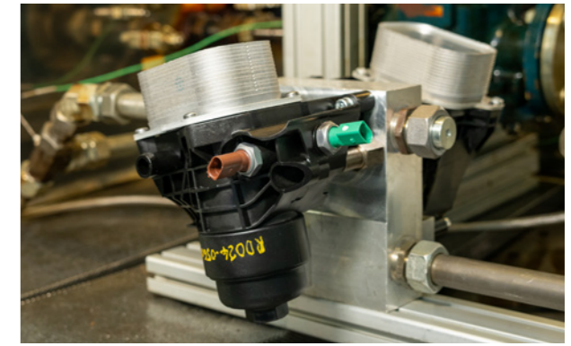
The oil filter modules are extensively tested on test benches.
